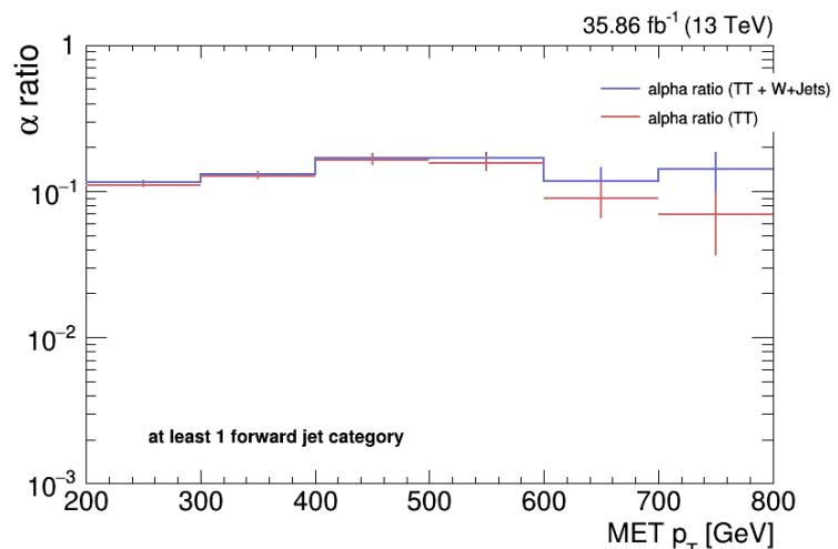
The shape of the distribution is obtained from the data in the CR and corrected by alpha, which is bin dependent.
