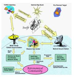
Within seconds of detecting a burst, the spacecraft will "swiftly" and autonomously repoint itself to aim the XRT and UVOT at the burst to enable high-precision X-ray and optical positions and spectra to be determined.
