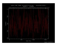
Selected time intervals are saved as GTI filters, and can be applied to the event file with XSELECT.
