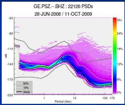
Comparison of the PSDs at selected frequencies for two hard rock based observatories, for CH.GIMEL in Switzerland and for Piszkéstető. The latter can be seen to be less noisy and significantly more stable.
