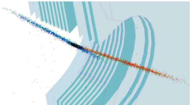
As the beam passes through LHCb, interactions with gas allow the experiment to measure the full beam profile. In this diagram, neon gas, beam 1 (blue) and beam 2 (red) are measured by the surrounding VELO detector.
