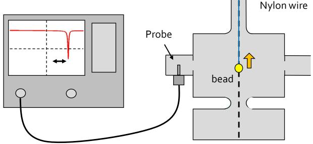
If the perturbing object (bead) is a perfectly conducting sphere the values of the form factors are:
