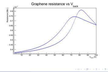
Since we would like to deplete the silicon below graphene we tried to obtain the Dirac point sweeping the top contact and the back together, while maintaining an offset between the two of:  $V_{back}-V_{top} = 20 \text{ V}$  corresponding to the one to assure depletion.
