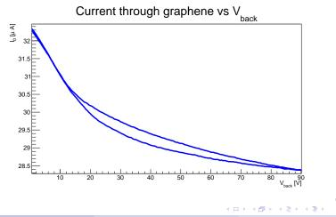
Using a different approach (sweeping both the top and the back contacts) we found 5 G-FETs that showed a clear Dirac point on the chip given in two interesting cells (cell 7 and cell 8). Not all G-FETs of the sample given have been connected since two cells with graphene are under the clamp or so near to it to make them unreachable with the needles of the probes.
