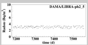
Time behaviours of the environmental radon in the installation (i.e. after the Supronyl), from which in addition the detectors are excluded by other two levels of sealing!
