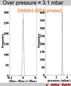
NO DM-like modulation amplitude in the time behaviour of external Radon (from which the detectors are excluded), of HP Nitrogen flux and of Cu box pressure
