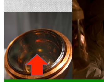
Second upgrade on Nov/Dec 2010: all PMTs replaced with new ones of higher Q.E.
