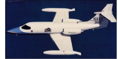
To avoid IR absorption in lower atmosphere, instruments were placed in aircrafts
