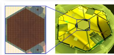
Figure 7: Prototype TES microcalorimeter array (left) and its supporting wafer (right) (NASA/Goddard)
