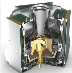
Figure 6: X-IFU Focal Plane Assembly (SRON)
