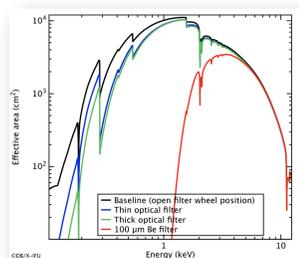
Figure 3: Athena/X-IFU Effective Area with 4 different positions of the filter wheel. Responses matrices are available at <http://xifu.irap.omp.eu>
