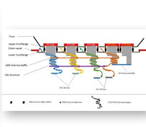
Figure 11: X-IFU cryoflange interfaces (CNES)
