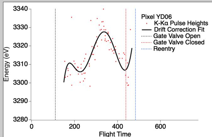
Filtered data from a single pixel during flight, prior to the correction for time varying gain, alongside the best fit curve used for drift correction.
