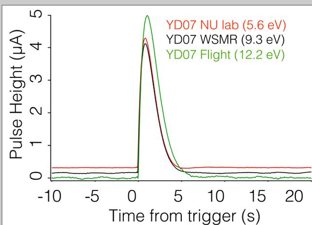
Pulses from one Micro-X pixel, measured in the lab, during preflight testing at WSMR and during flight. Baseline oscillations from the simultaneous operation of both science chains are visible in the latter two traces.
