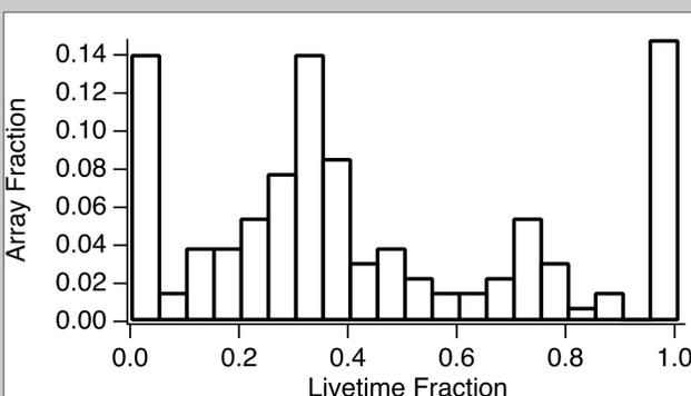
This plot depicts the stability of the array during the science portion of the Micro-X flight. One of the eight columns was live for the entire observation and another was inactive for the entire observation, with a spread of values on other columns.
