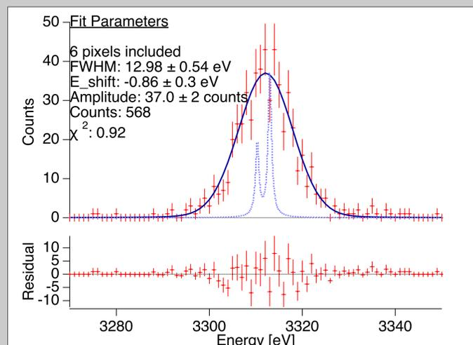
Flight spectrum from 6 coadded pixels in the Micro-X detector, measured from the internal calibration source.
