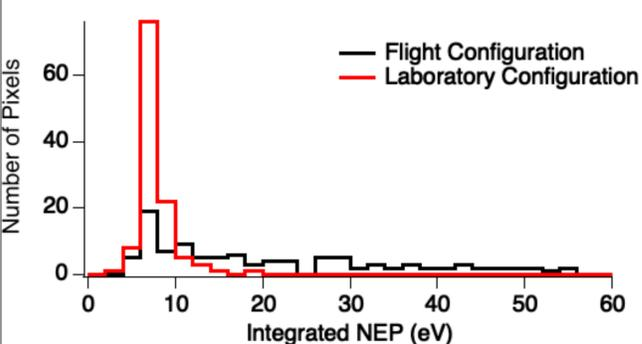
Depicted here is a histogram of the integrated NEP within the Micro-X TES array during laboratory (red) and field testing (black). The laboratory measurement was conducted in two parts, sampling each half of the array separately while the measurement from the field in flight configuration read out both sides simultaneously.
