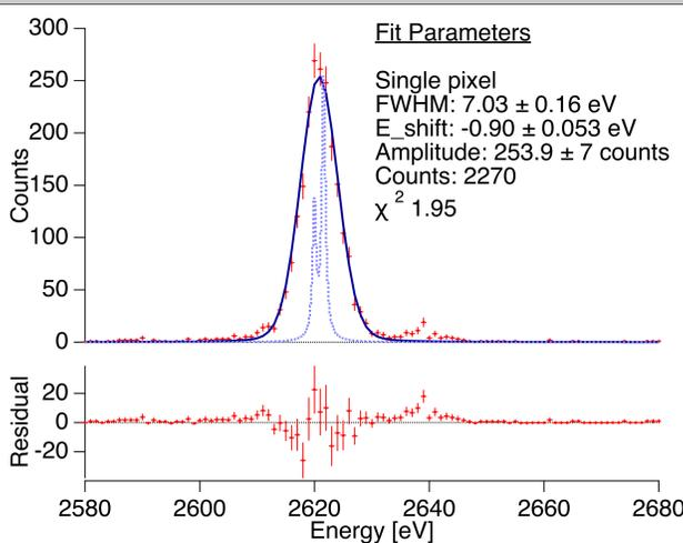
Spectrum from a single pixel in the Micro-X detector, measured while observing the internal calibration source over an extended continuous period. The instrument was in flight configuration with both sides of the readout operating.
