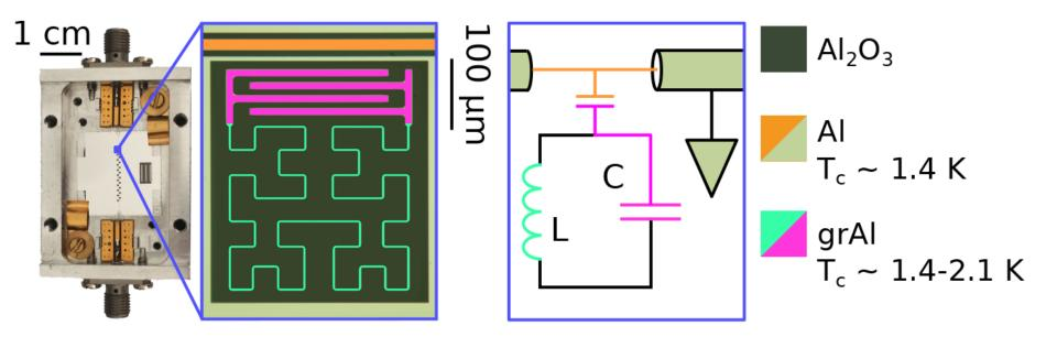
Granular aluminum (grAl): a low-loss, gaptunable composite material
