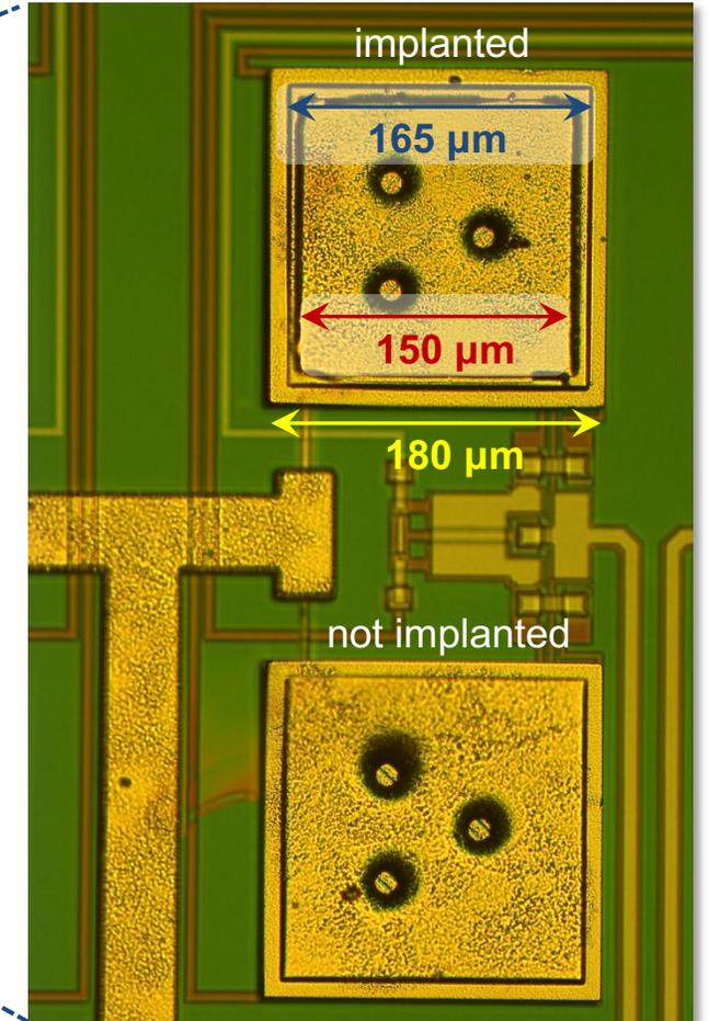
*Microscope image of implanted MMC channel*
