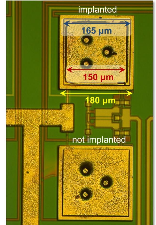
*Microscope image of implanted MMC channel*
