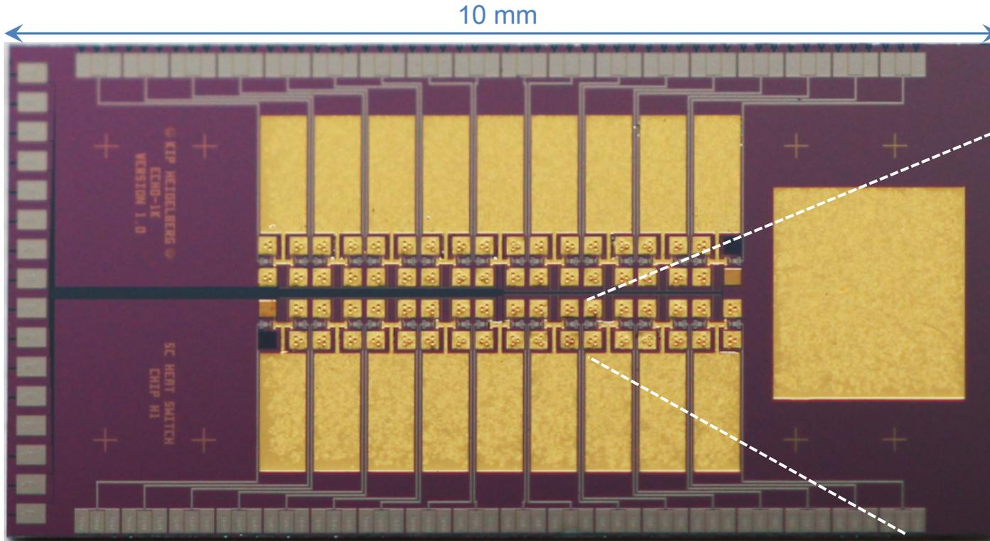
32 gradiometric channels → 64 MMC pixels
