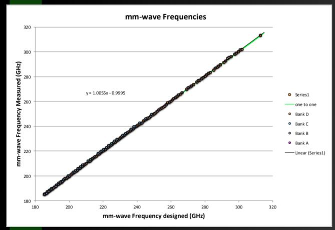
We have now demonstrated an ability to produce the resonators at the design frequency over the full range of frequencies
