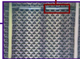
Each grid-square has **two interleaved phased antenna array sets** of orthogonal polarizations.
