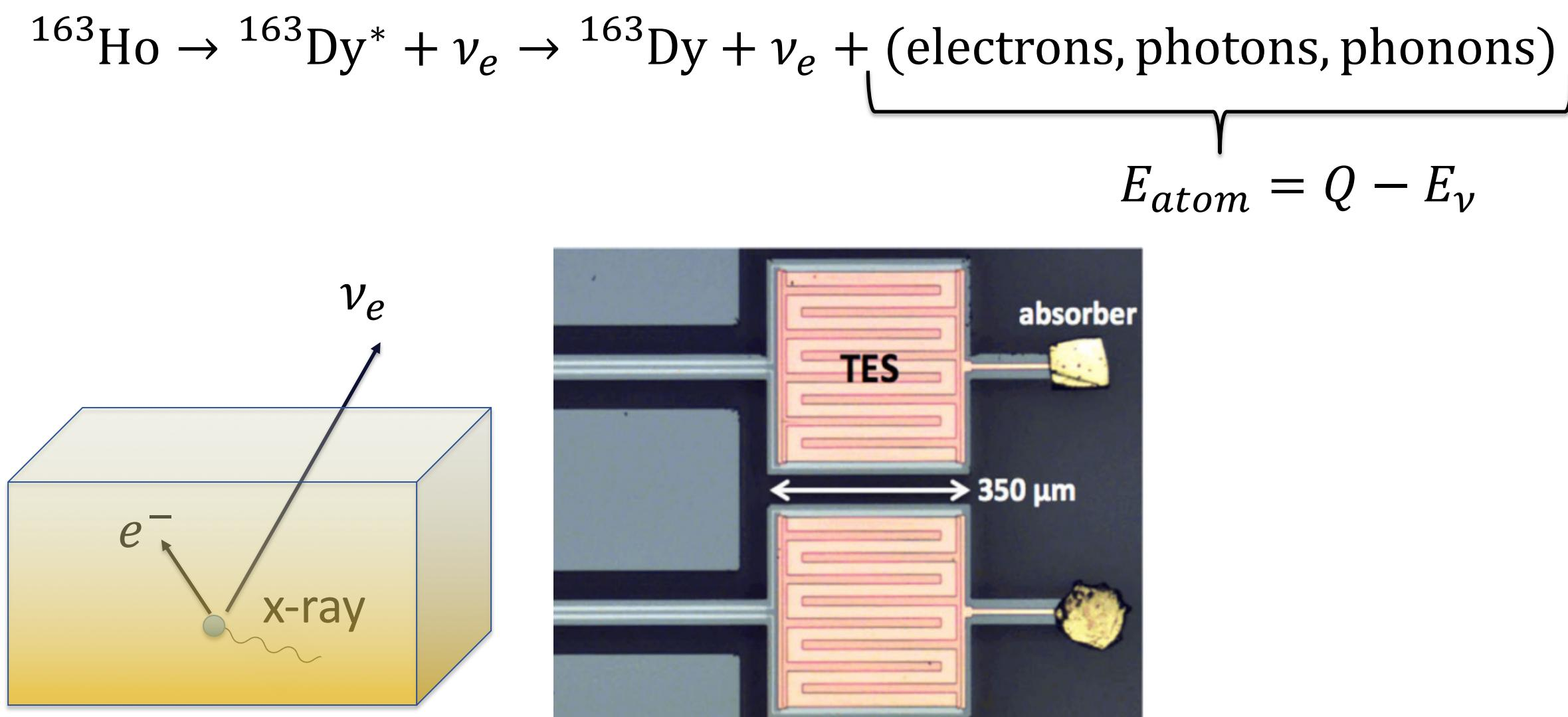
The advantage of a calorimetric measurement (conceptual drawing at left): no need to know fluorescent yield, because all atomic decay energy is thermalized and measured as heat. Microcalorimeter Transition Edge Sensors (right) provide the required energy resolution (< 10 eV FWHM at 2 keV) for a kinematic neutrino mass measurement.
