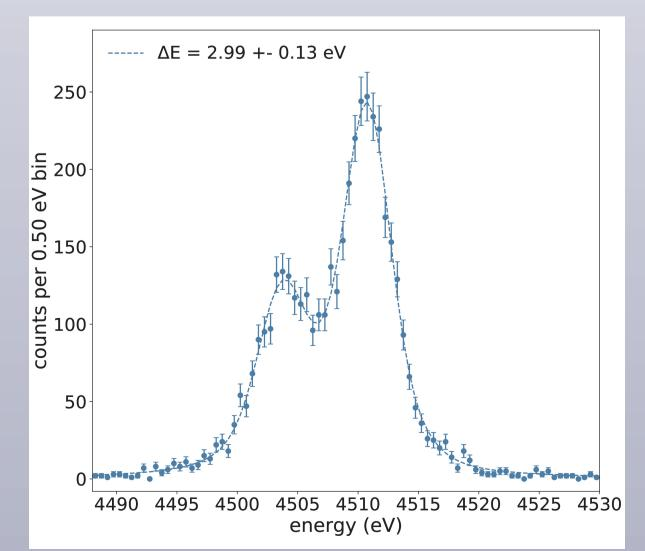
At  $f_r = 500$  kHz, average max slew rate of Ti K $\alpha = 0.44$   $\Phi_0$ /sample, no correction is needed. The detector's energy resolution was  $\Delta E = 2.99 \pm 0.13$  eV FWHM.
