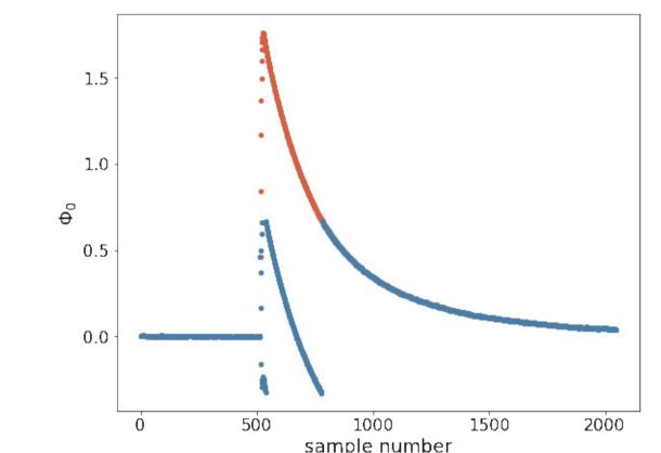
Standard unwrapping: if consecutive samples differ by a phase shift of  $>\pi$ , shift the data down by  $2\pi$ . If they differ by  $<-\pi$ , shift up by  $2\pi$ . Left: raw data after demodulation. Right: before (blue) and after (red) unwrapping. The max phase shift is  $<\pi$ , so demodulation succeeds.
