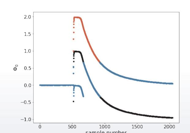
Biased unwrapping: For phase shifts  $>\pi$ , standard unwrapping may shift data in the wrong direction (black trace). But, during a pulse the largest phase shift occurs on the rising edge. So, we "bias" the unwrapping algorithm: if the ratio of falling edge to rising edge slew rate is X, shift differences of  $>2(1-X/2)\pi$  by  $-2\pi$ , and differences  $<-X\pi$  by  $+2\pi$ . The effective slew rate limit is  $(1-X/2)\Phi_0 f_r/2M_{in}$ .
