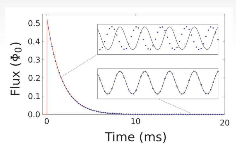
For an unknown signal, it's impossible to distinguish a phase shift of  $> \pi$  from  $< -\pi$ . So, the nominal limit on current slew rate (in A/s) between samples is:
