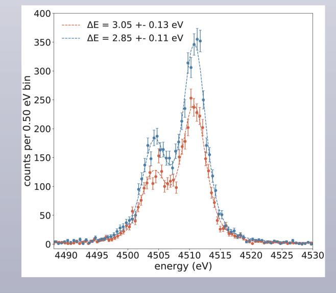
Blue:  $f_r = 250$  kHz, avg. max slew rate =  $0.8 \, \Phi_0$ /sample,  $\Delta E = 2.85 \pm 0.11$  eV FHWM. Red:  $f_r = 500$  kHz data downsampled to 250 kHz,  $\Delta E = 3.05 \pm 0.11$  eV.
