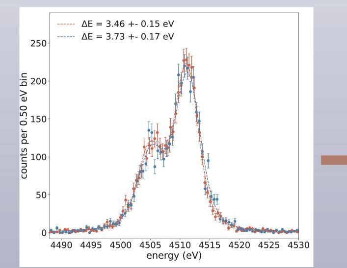
Blue: fr = 125 kHz, avg. max slew rate = 1.36  $\Phi_0$ /sample,  $\Delta E = 3.73 \pm 0.17$  eV. Red: data downsampled from 500 kHz to 125 kHz,  $\Delta E = 3.46 \pm 0.15$  eV, suggesting degradation can be accounted for primarily by arrival time effects induced by undersampling the rising edge.
