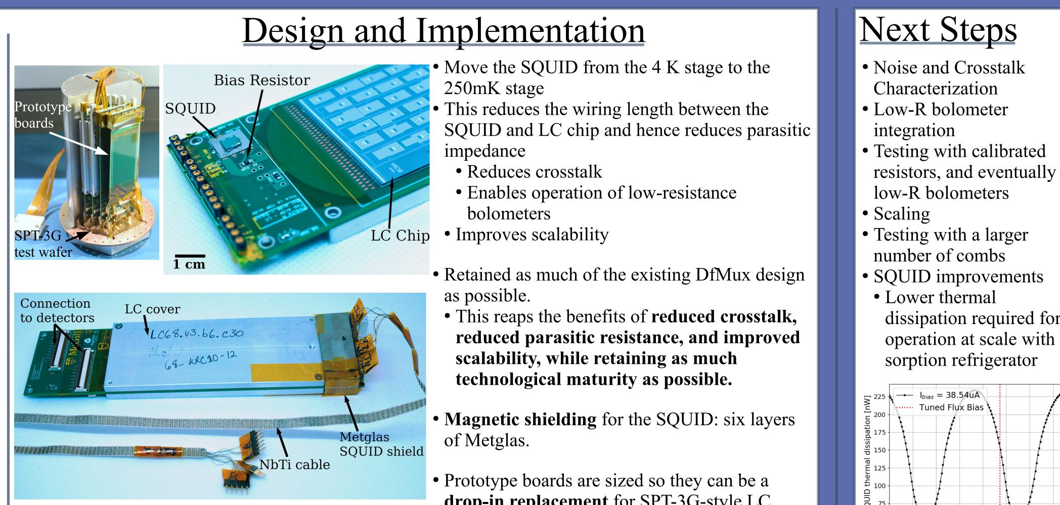
•We have designed and implemented a readout with the SQUID next to the LC • Reduced wiring length  $\rightarrow$  reduced parasitics
