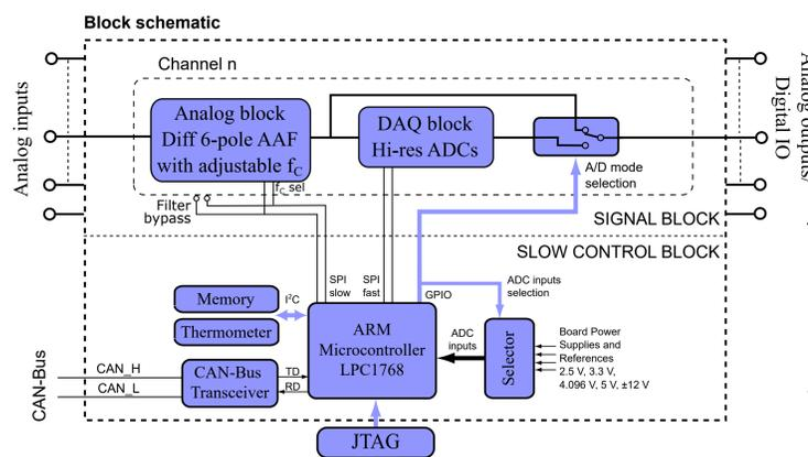
Figure 4: Block schematic of the DAQ board for CROSS
