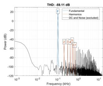
Figure 6: Measurement of THD with a 100 Hz sine (cut-off at 2.4 kHz) using internal DAQ (32 ksp/s)
