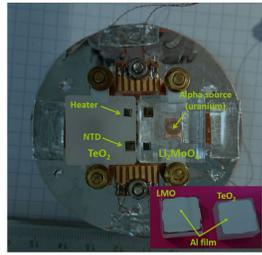
Figure 1: Photo of CROSS prototype setup
