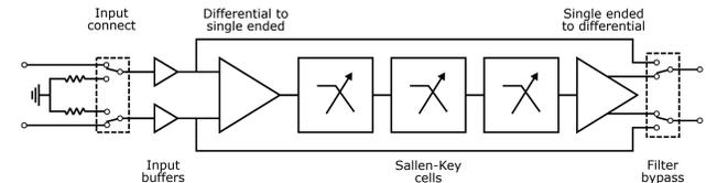
Figure 5: Analog filtering block with programmable cut-off frequency
