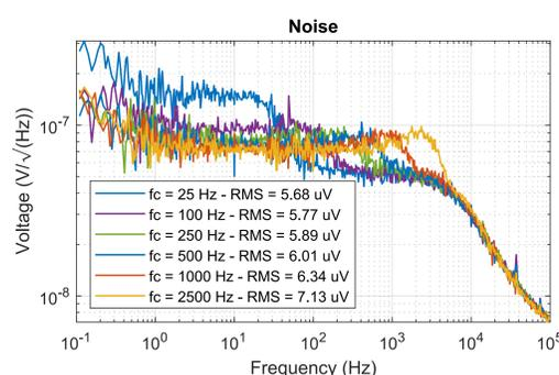
Figure 9: Analog noise spectra at different cut-off frequency settings
