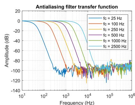
Figure 8: Analog filter transfer function at different cut-off frequency settings
