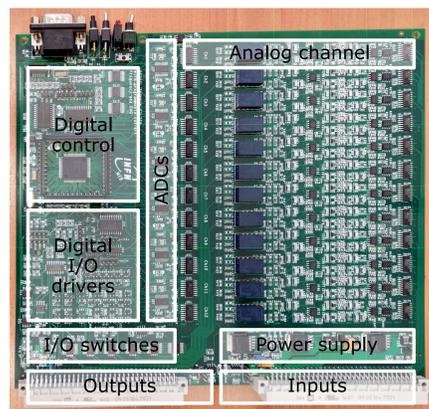
Figure 3: Photo of the antialiasing filter and DAQ board for CROSS
