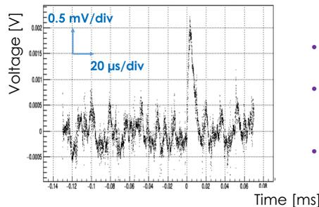
Output waveform of STJ's signal amplification
