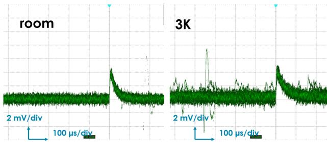
Output waveform test signal amplification ( $Q_{in} = 0.49$  fC)
