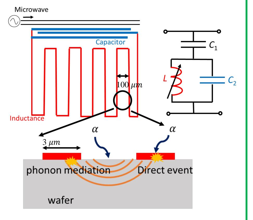
(top) Schematic drawing of Lumped element Kinetic Inductance Detector (LeKID) and Equivalent circuit of LeKID. (bottom) Alpha particles emitted from Am241 enter the top side of the device.
