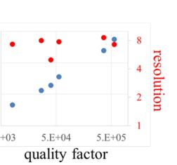
The higher Q resonator has longer pulse but has equivalent energy resolution.
