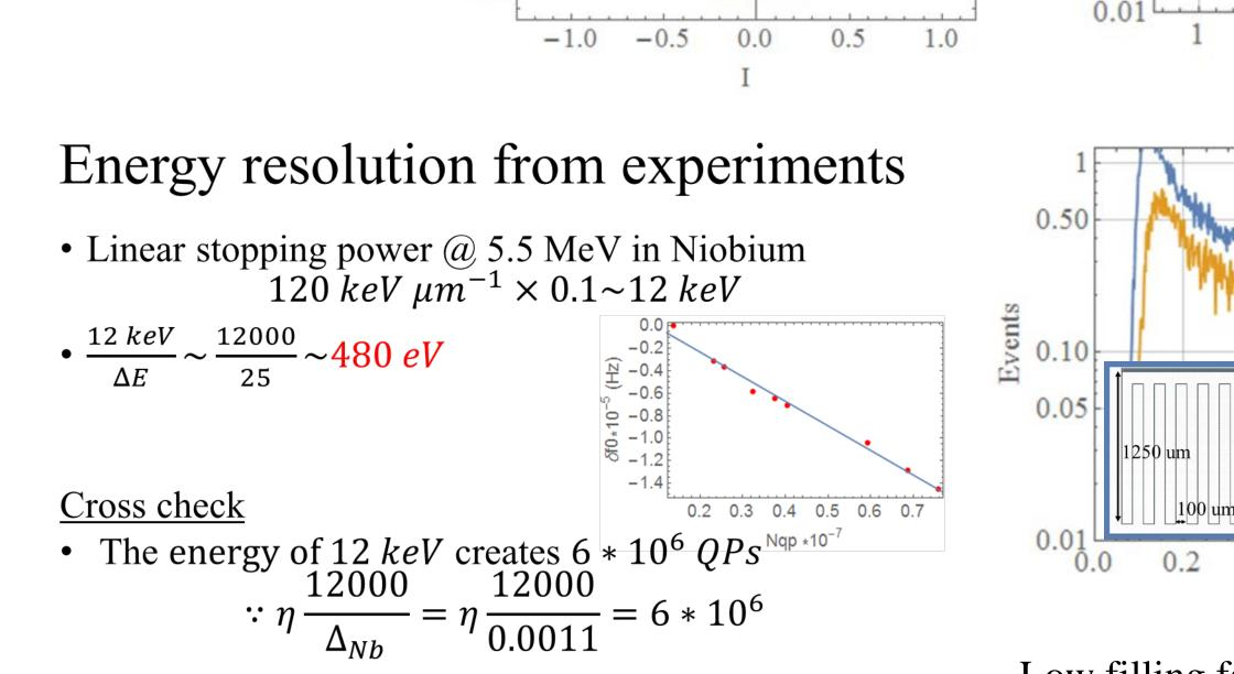
• The maximum pulse height indicates that  $5 * 10^6 QPs$ are excited in the resonator.
