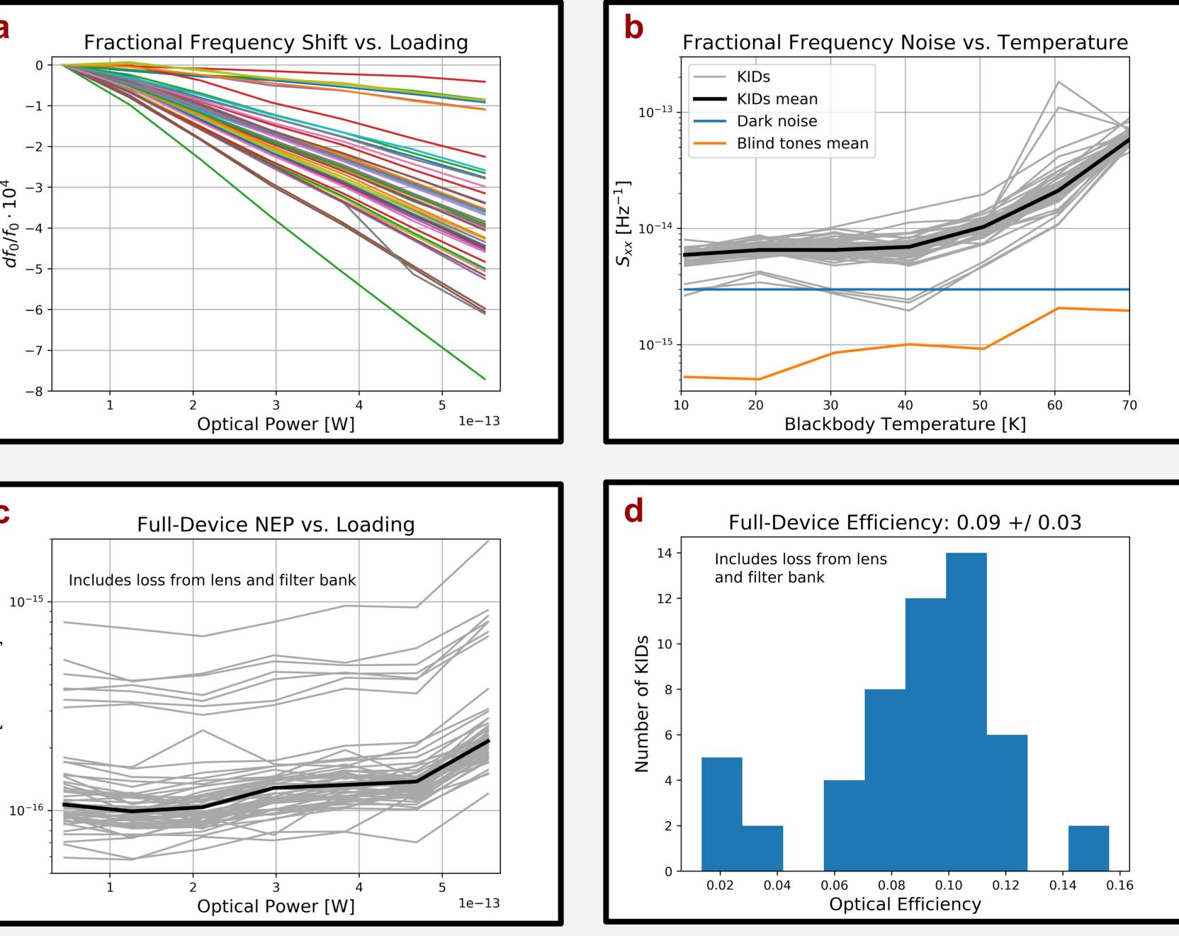
From the fractional frequency shift vs. loading (a) we determine device responsivity. Fractional frequency noise (b) is estimated by finding the white noise level of 200 s timestreams above the optical chop frequency of ~1 Hz. Dark noise measured on the same device is lower than Sxx we measure here, as are several blind tones placed throughout the band, indicating that we measure photon noise.
