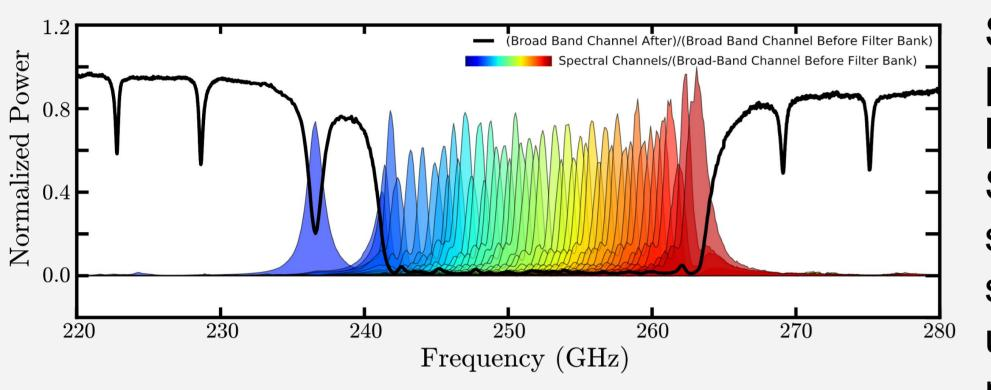
Spectroscopy from 200-300 GHz [2] is sensitive to far-IR emission lines from early galaxies. Future SuperSpec devices will enable sensitive multi-object spectrographs and integral field units suitable for line intensity mapping at high redshift.
