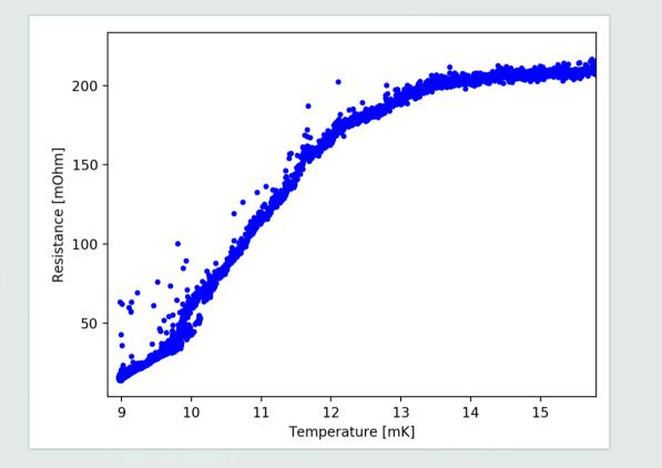
The resistance variation of the TES as a function of the temperature is shown in the Figure. The resistance value was measured with a DC-SQUID based read-out system. The tungsten TES showed a normal-tosuperconducting transition between 9 mK and 14 mK.
