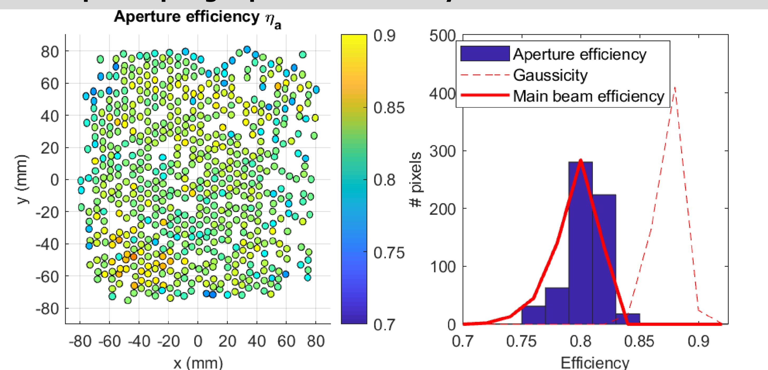
The aperture efficiency is the plane wave coupling at telescope, point source on sky. Gaussicity is the coupling to an ideal Gaussian beam, in plane of measurement. The main beam efficiency (extended source) is calculated from the on sky beam pattern overlap integral, using a source of radius  $1.22\lambda/D$ . Yield ~80% of pixels measured.
