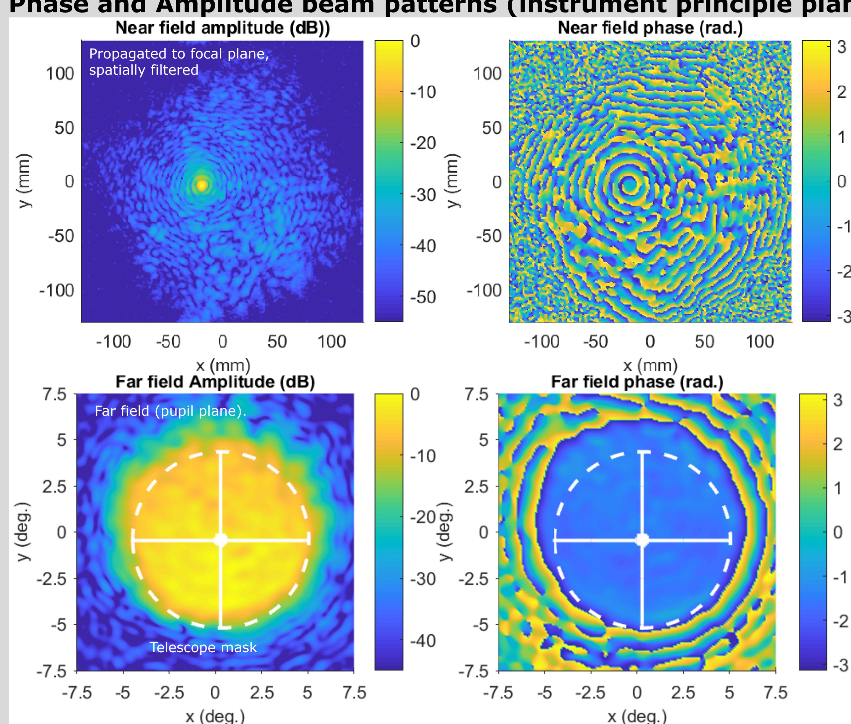
Top: measured phase and amplitude beam patterns spatially filtered and propagated 30mm to focal plane. Bottom: far field beam pattern calculated from the measurement, an image of the system pupil. A telescope model is generated by applying a mask, indicated in white.
