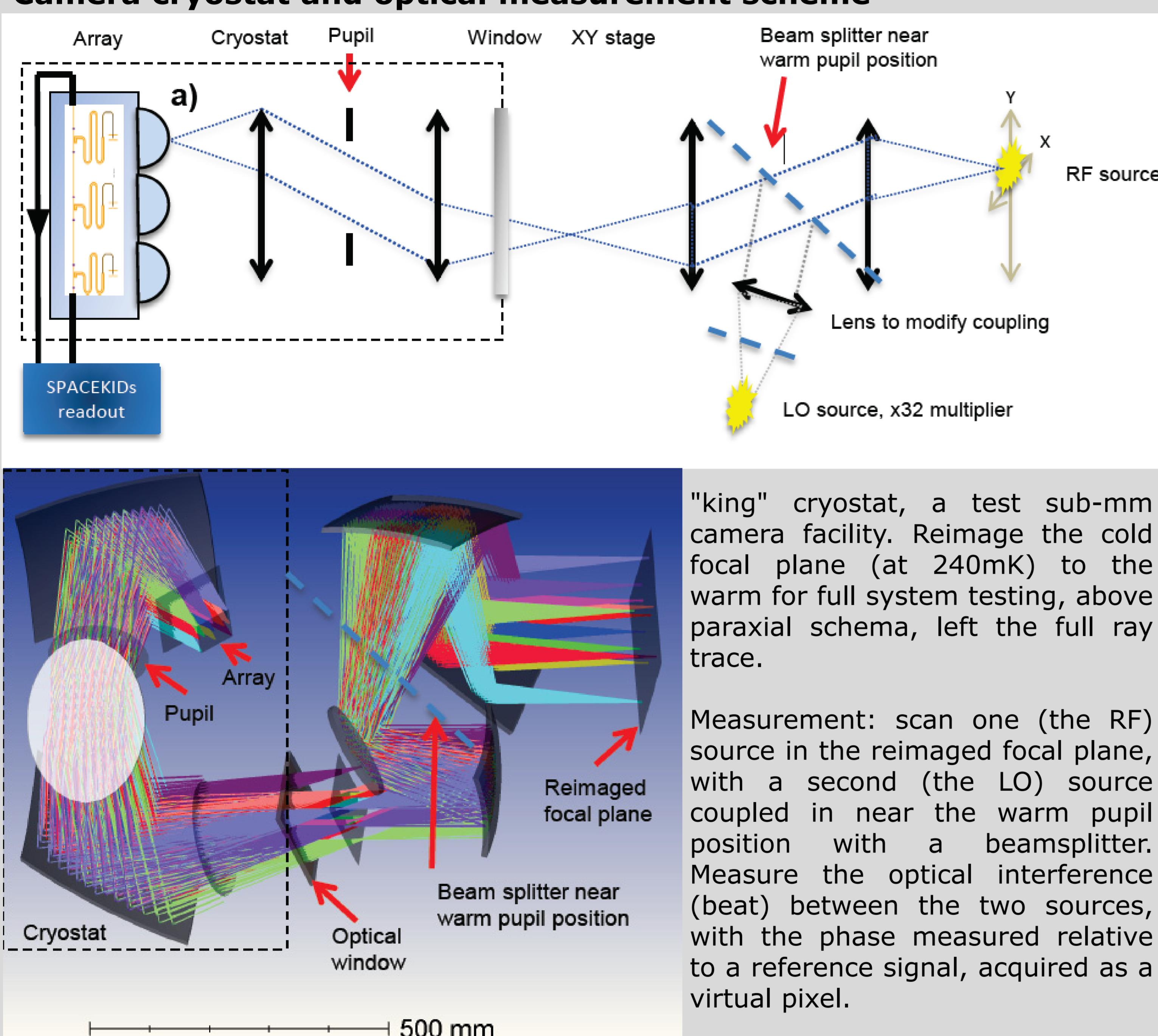
"king" cryostat, a test sub-mm camera facility. Reimage the cold focal plane (at 240mK) to the warm for full system testing, above paraxial schema, left the full ray trace.
