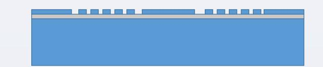
Pattern phononic features using electron beam lithography. Etch into the device layer and stop on the buried oxide.
