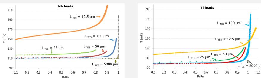
$T_{c,i}$  and  $T_{c,eff}$  plotted as a function of  $R/R_n$ . The long 5000  $\mu\text{m}$  length TES defines the  $R/R_n = 1$  limit (dashed line) based on the value of the measured sheet resistance  $R_n$ .
