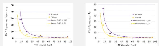
The width of the measured transition curves defined as  $T_{c,eff}(R/R_n = 0.8) - T_{c,eff}(R/R_n = 0.1)$  scales as  $1/L^2$  (plot left side). Also the  $T_{c,eff}$  at 0.5  $R_n$  showed the  $1/L^2$  scaling (plot right side). The  $1/L^2$  scaling clearly indicates weak link behavior.
