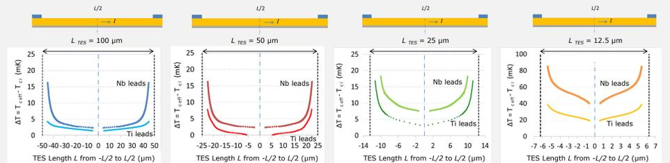
By assuming the proximity effect is increased near the leads and decays with distance away from the leads to a minimum at  $L/2$ , we converted the  $R/R_n$  value to distance units. The plots above show the difference between  $T_{c,eff}$  and  $T_{ci}$  as a function of TES length displayed from  $-L/2$  to  $L/2$ .
