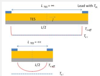
To determine the magnitude of the effect of the leads on the intrinsic transition curve of our TiAu bilayer, we have designed test structures with different TES lengths ( $L$ ). We produced two sets of test structures, one set with Nb leads, one set with Ti leads.
