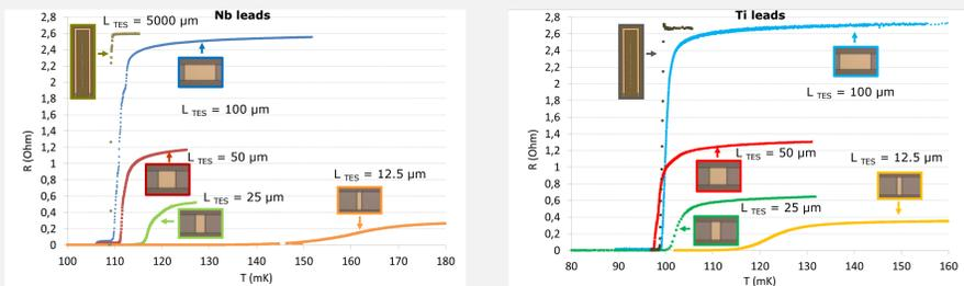
$R(T)$  curves of test structures with 35/200 nm TiAu bilayer TESs. On the left side plot TESs were connected with Nb leads, on the right side Ti leads.
