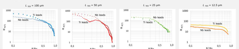
Plots of  $\alpha$  versus  $R/R_n$  for all the TES lengths to compare Nb with Ti leads. Transition parameter  $\alpha = (T/R)(dR/dT)$
