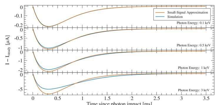
Figure 6: Pulse shape comparison between simulation and TES small-signal model [3] for different photon energies. The pulses match very well for small energies. For higher energies they start to deviate as expected due to the non-linearities in the system.
