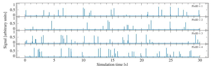
Figure 3: Individual signals of a four pixel configuration during a 30 seconds simulation with random impacts, using the current best estimate X-IFU pixel parameters. Currents are flipped and normalized.
