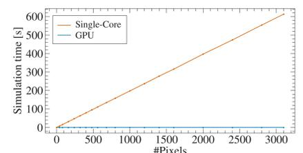
Figure 4: Run time comparison between single-core and GPU accelerated version on an Nvidia GeForce GTX 1080 Ti for different array sizes simulated for one second each.
