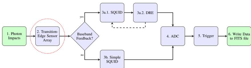
Figure 1: Data flow in *xifusim*. A list of photon impacts is propagated to the TES array where the pixel responses are calculated. Their signal is amplified in a set of SQUIDs, either using a simple, fast SQUID model or a model implementing the nonlinear SQUID response and baseband feedback. An Analog-Digital-Converter maps the measured current into a digital signal which is passed to a trigger that detects the individual pulses in the datastream and writes them to the output file.
