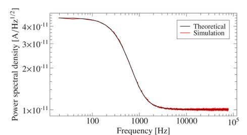
Figure 5: Comparison between predicted and simulated noise levels. Included noise sources are Johnson noise of the TES and load resistor, thermal fluctuation noise and noise from the bias line.
