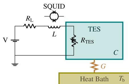
Figure 2: The TES model we implement in our software, consisting of the Thevenin-equivalent representation of the bias circuit coupled to the TES.
