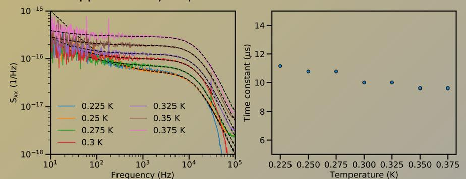
Fig 5: Left: Fits to the noise spectrum of a SuperSpec detector ( $T_c = 1.5$ ). Right: The extracted  $\tau_{qp}$  as a function of array temperature.  $\tau_{qp}$  is found to be roughly independent of the array temperature for the temperatures measured here. Ringdown time is 1.7  $\mu\text{s}$ .
