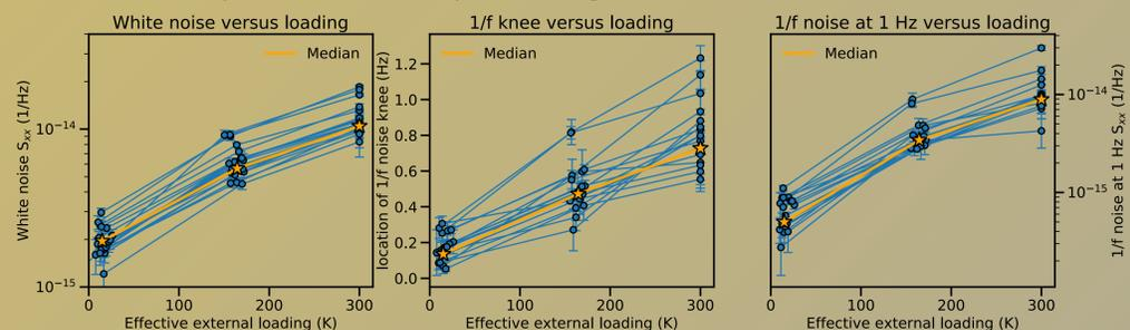
Fig 4: Noise versus loading for 37 SuperSpec detectors. 1/f knee is the frequency at which half of the noise is 1/f and half is white, frequency independent, noise. Principle component analysis has been performed to remove common mode noise.
