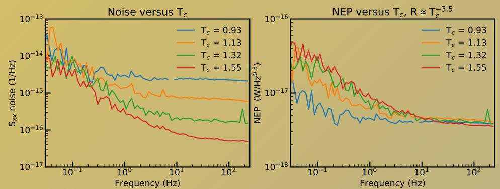
Fig 3: Plots showing the effect of  $T_c$  on the 1/f noise level for SuperSpec detectors. Left: The raw noise data in  $S_{xx}$  units. Right: Hypothetical NEP achieved assuming that the responsivity of the detectors goes as  $T_c^{-3.5}$  (empirically observed).
