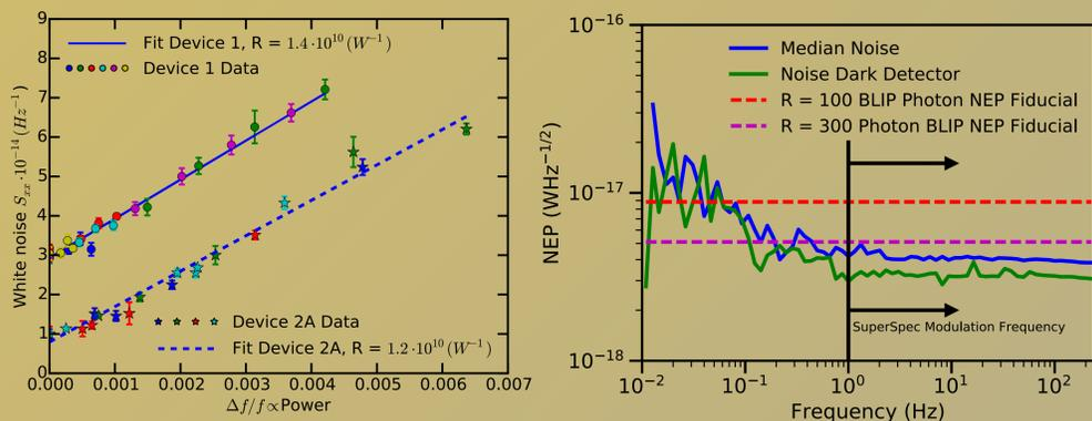
Fig 2: Left: Measured responsivities for two spectrometers using coherent source method (Hailey-Dunsheath et al. 2015 LTD Proceedings). Each different color symbol represents a different detector. Right: NEP PSDs for SuperSpec detectors.
