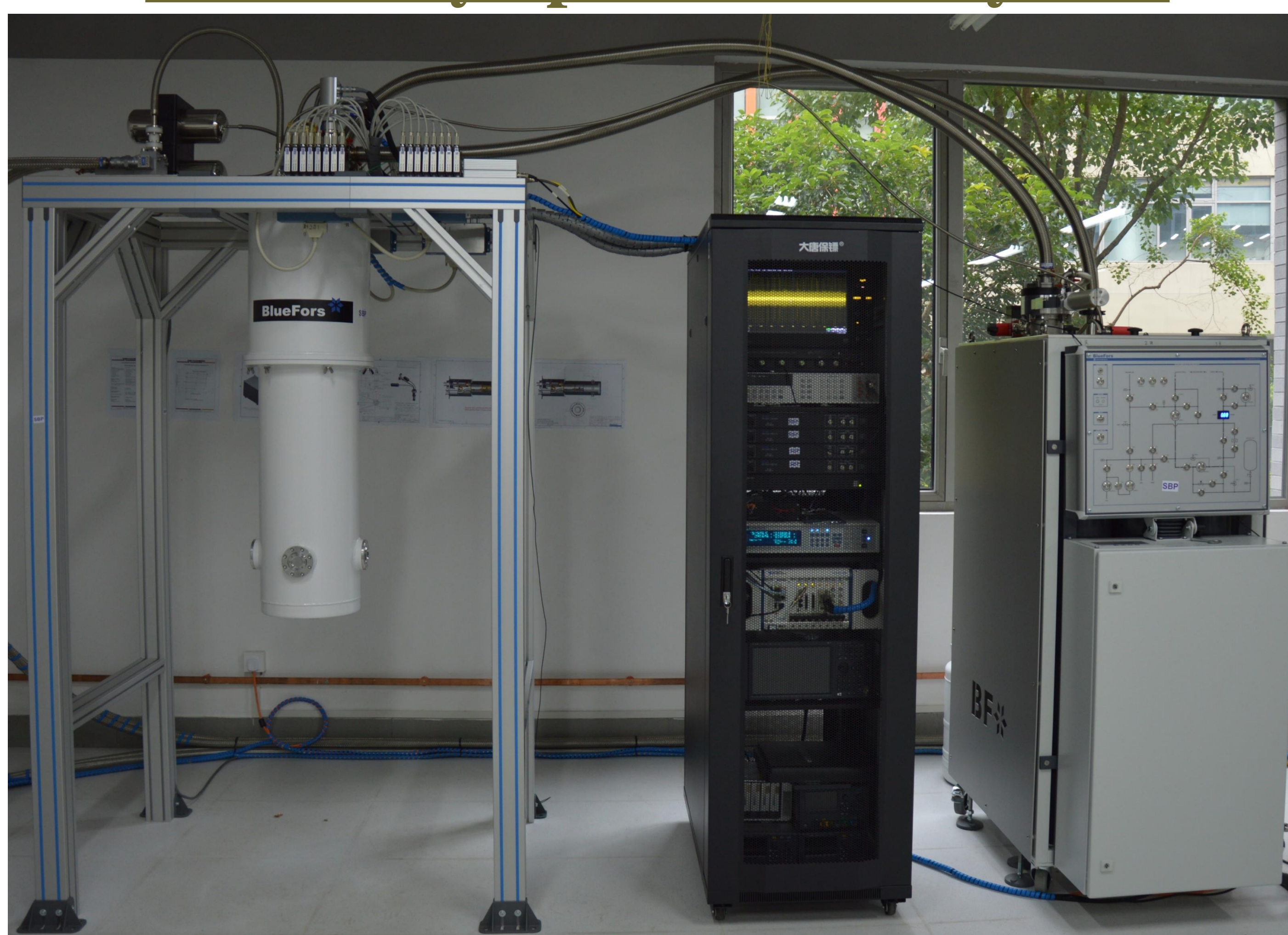
Fig1: Photo of the TES X-ray spectrometer, the dilution refrigerator can reach down to 21mK, the SQUID and data acquisition (DAQ) system allow 32 pixels readout simultaneously.
