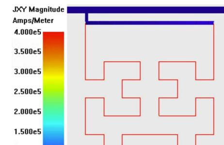
The lumped element condition is verified: the current is uniform in the absorber/inductor and null in the capacitor
