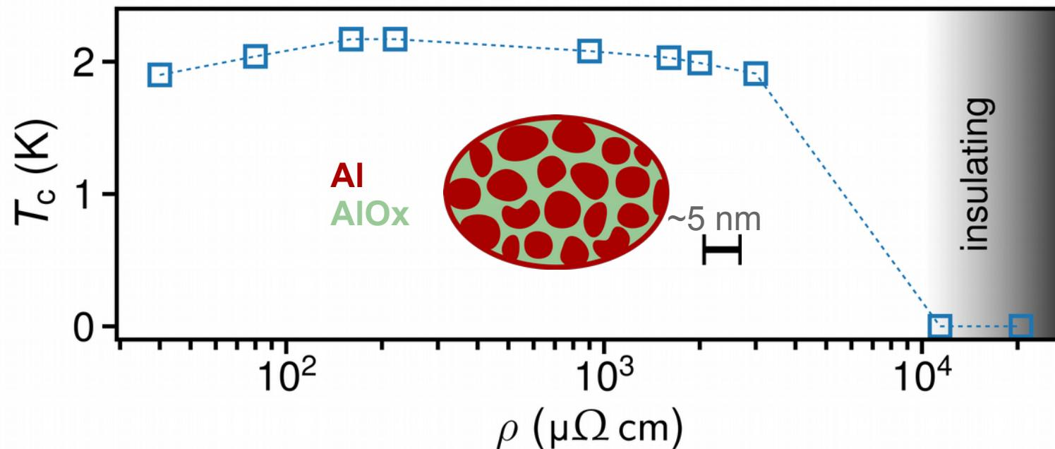
$\rho$  tunable by control of oxygen pressure during evaporation
