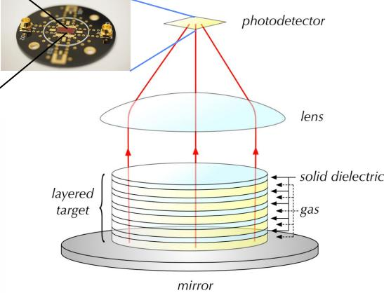
Key advantage of these detectors is low Dark Count Rate (DCR) and low-energy threshold. Depending on number of layers in target, and achievable DCR, reach of experiment could extend well beyond what is possible today
