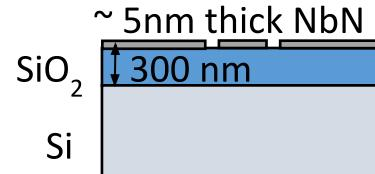
CPW, 300 nm center conductor width,
