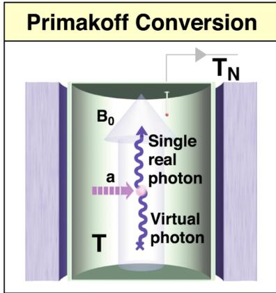
$$P \propto g_{a\gamma\gamma}^2 \frac{\rho_a}{m_a} B_0^2 V C Q$$
