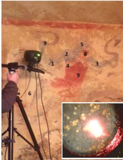
Commercial (ELIO XG-Lab) XRF system for in situ analyses
