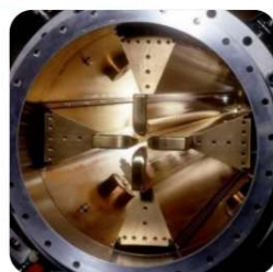
Linac 2 – 1990 200 MHz, p + 165 mA, 750 keV (build at CERN)
