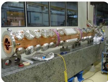
Linac 4 – 2007 352 MHz, p - 80 mA, 3 MeV (build at CERN)
