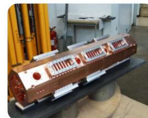
TRASCO (INFN) – 2003 352 MHz, p + 30 mA, 5 MeV (brazed at CERN)
