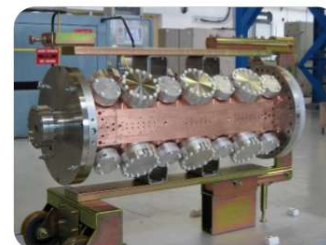
IPHI (CEA) – 2008 352 MHz, p + 100 mA, 5 MeV (Modules brazed at CERN)
