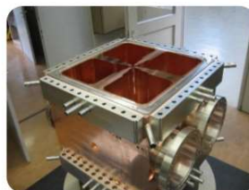
IFMIF (INFN) – 2010 175 MHz, d + 130 mA, 5 MeV (Prototype brazed at CERN)
