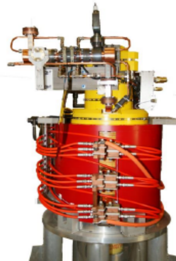
X-band klystron: provided by CERN
