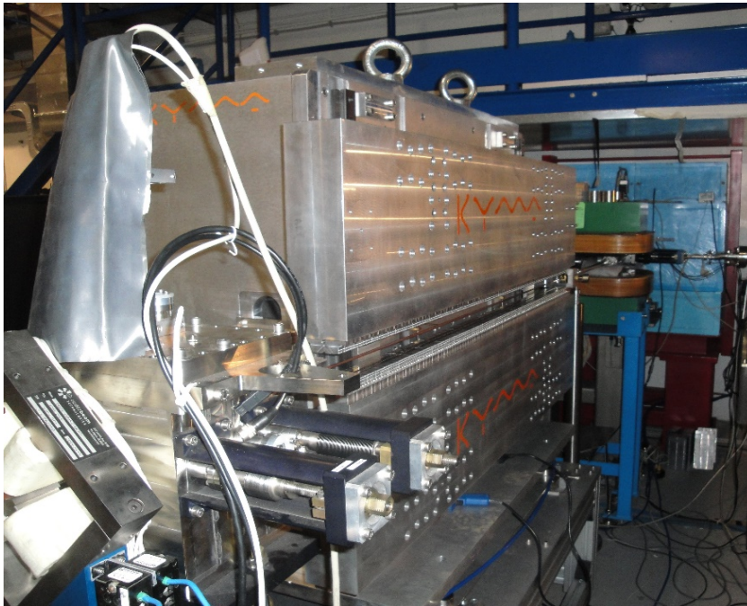
KYMA \Delta undulator at SPARC LAB: \lambda=1.4 cm, K1
