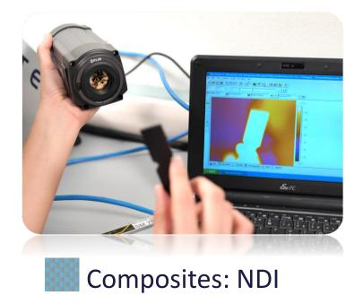
We rely on NDI techniques like Radiography, Tap Test, Thermography, Ultrasounds and Tomography to guarantee the quality of the structures we produce
