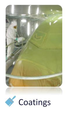
Aerospace and Defense more than any other require for special coatings to be applied before delivery, namely Painting, Flam Sprays, Aesthetic Film Foiling, Kapton, Tedlar, and many more
