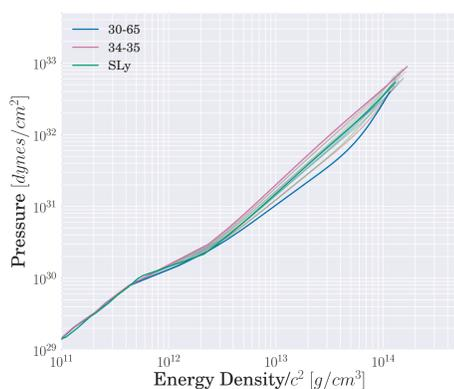
**Figure 1:** The EOSs for realistic crust models with nuclear parameters  $S_0 \in [30 - 34]$  MeV and  $L \in [30 - 70]$  MeV. SLy is characterized by  $S_0 = 32$  MeV and  $L = 46$  MeV. The 34-35 MeV and the 30-65 MeV EOSs are the upper and lower limits.
