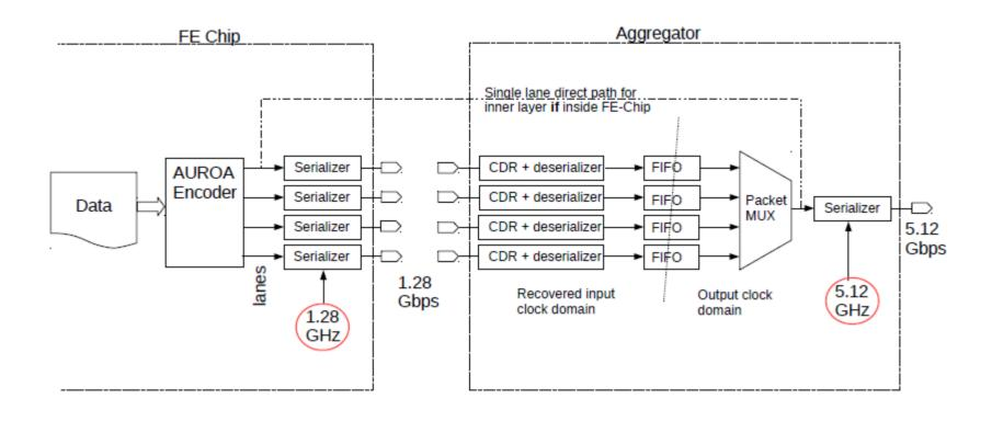
Aggregator chip from Pixel TDR Input 4 lanes (1.28 Gbps) from FE → Ouput 5,12 Gbps electrical connection
