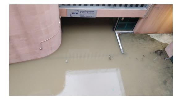
All Tier-1 doors are watertight Height of water outside: 50 cm Height of water inside: 10 cm (on floating floor) for a total volume of ~500 m<sup>3</sup>
