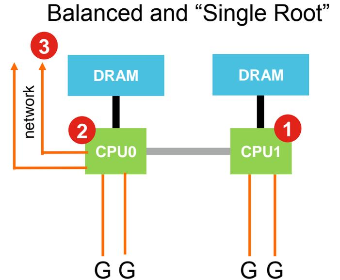
4 GPU systems are ideal for both HPC and AI. Minimal hops to network and from GPU-GPU
