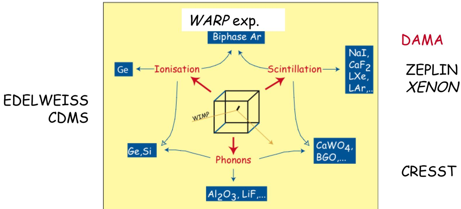
Simultaneous use of several detection mechanism allow better background rejection and better control of systematics
