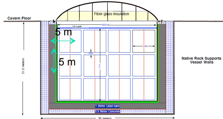
Inner containment vessel corrugated Stainless Steel or Invar, Inner wall dimensions are fixed. Green is 3/4 inch plywood backing. Red is capping material for foamglas insulation. Dark gray is 1 meter thickness of foam glass insulation which is also used as secondary containment of LAr. Outer blue is reinforced concrete, 0.5 meter at base to support hydroststic head and vessel pressure loads... Vertical concrete fills gaps so that vessel walls are supported by native rock.
