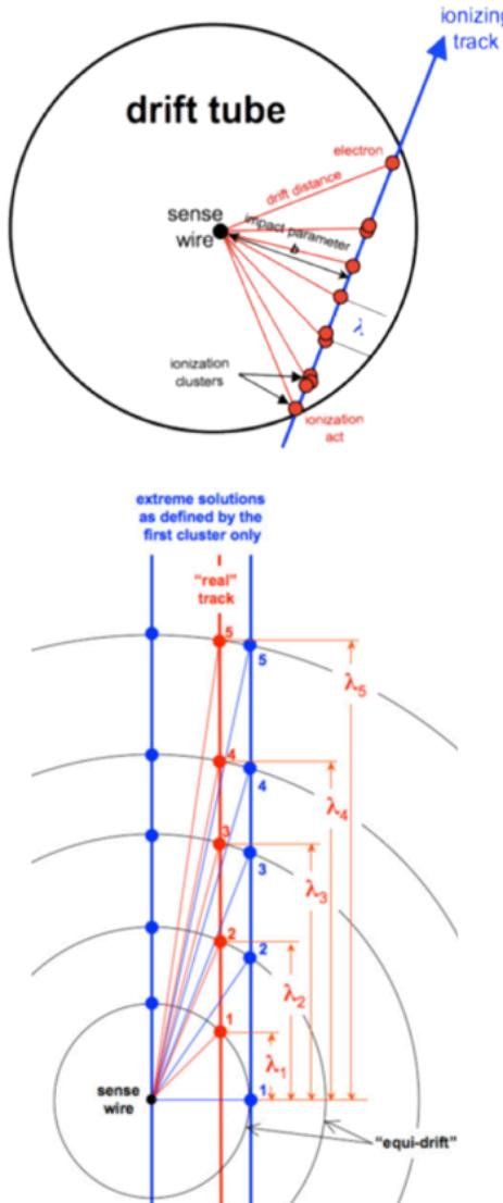
From the **ordered sequence of the electrons arrival times**, considering the average time separation between clusters and their time spread due to diffusion, reconstruct  $\{t_i^{cl}\} \quad i = 1, N_{cl}$  probable sequence of electrons drift times:
