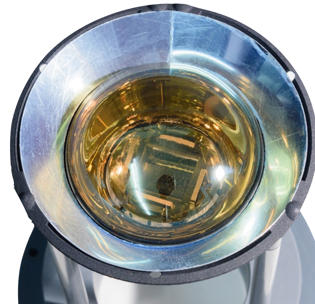
Reflector with PMT in test support structure
