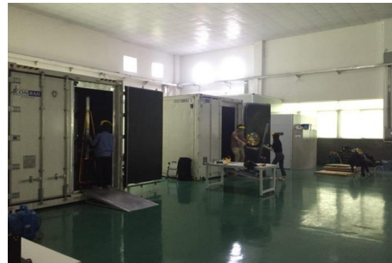
Batch test of 72 PMTs in two containers
