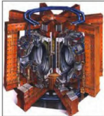
JET, the Joint European Torus, is the world's largest operational magnetic confinement plasma physics experiment, located at Culham Centre for Fusion Energy, Ox, UK.
