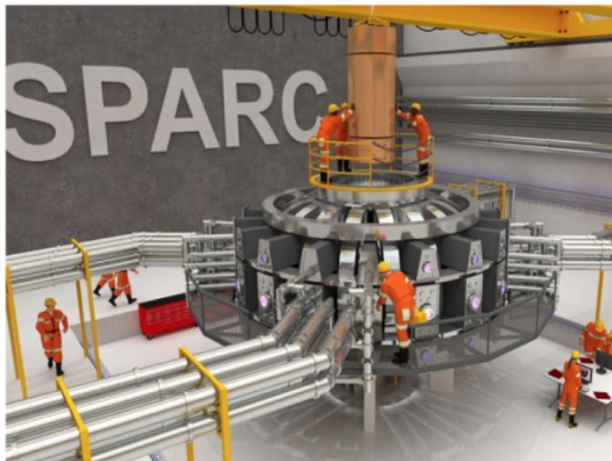
Visualization of the proposed SPARC tokamak experiment. Using high-field magnets built with newly available high-temperature superconductors, this experiment would be the first controlled fusion plasma to produce net energy output.
