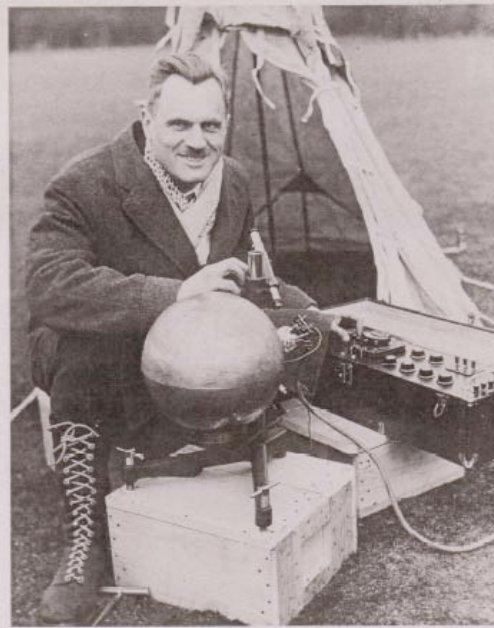
Fig. 4. Compton with the special ionization chamber which he designed and used for his world-wide cosmic-ray survey during 1931-33, which proved that cosmic rays are charged particles.
