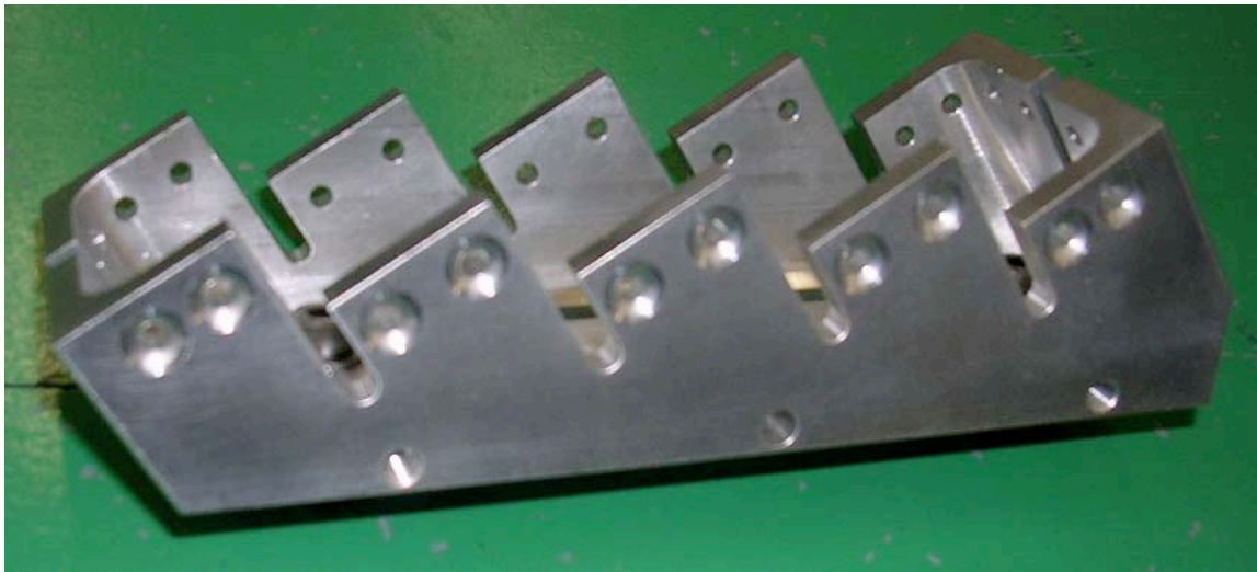
Rear closure & fixation by complex machined part riveted to alveolar
