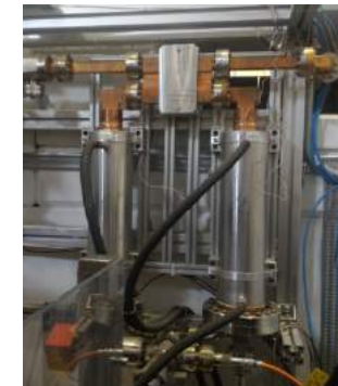
Pulse compressor: provided by CERN
