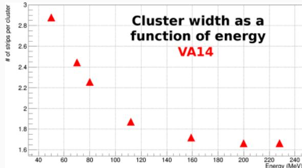
Figure 4: Cluster width as a function of energy for the two VAs
