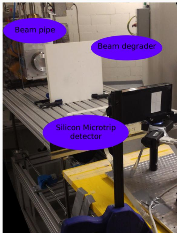
*Goal of the test: use low energy beam data to investigate possible saturation effects of the electronics*
