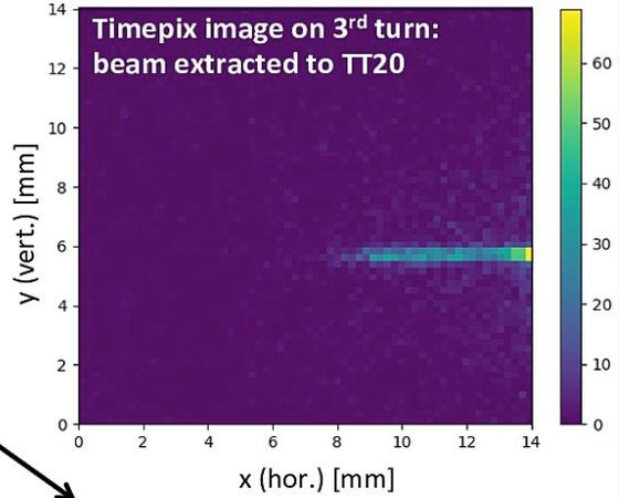
channelled beam extracted to TT20 at ZS
