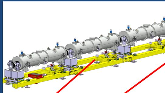
5 Electromagnetic septa mounted on the same support
