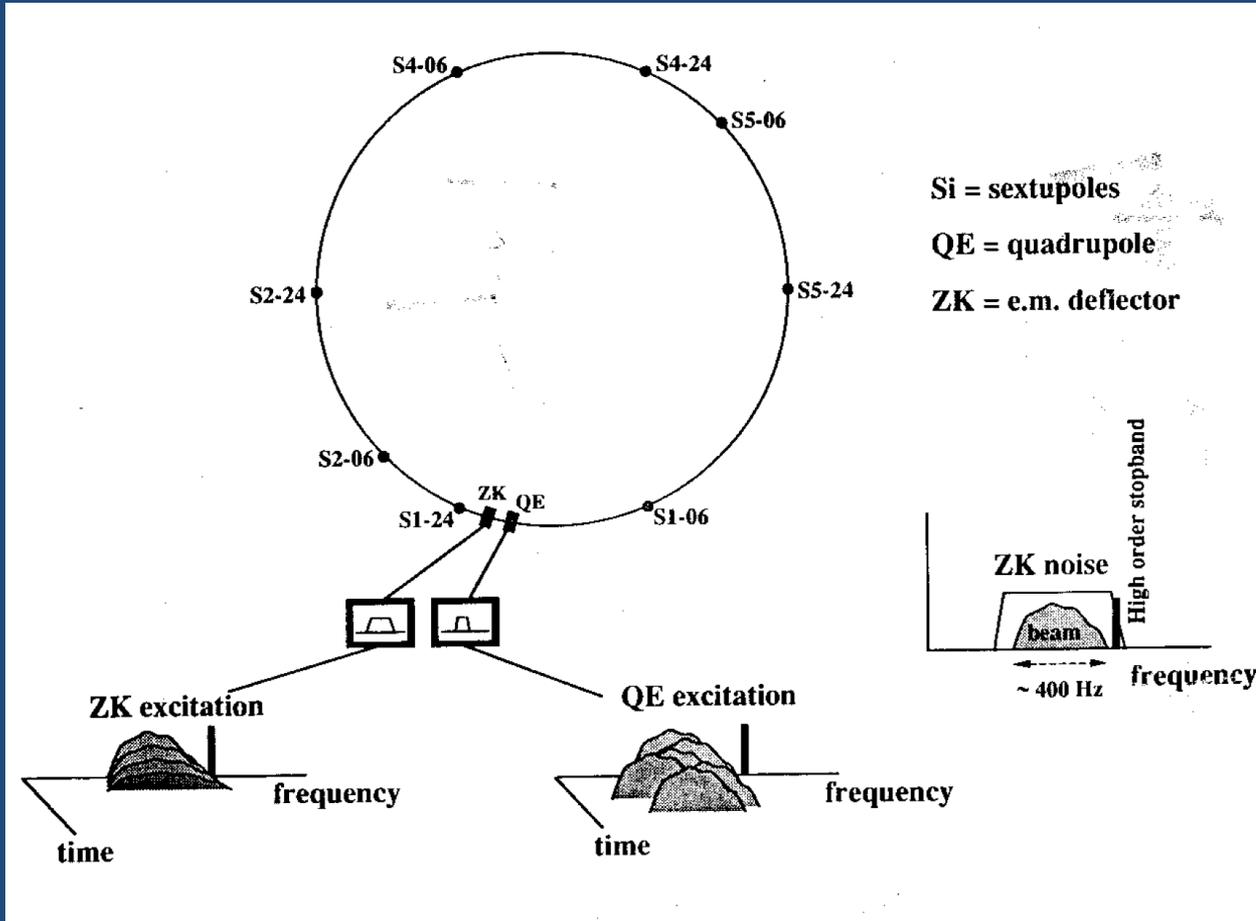
An electromagnetic device (ZK) could be used to induce random deflections in the circulating beam and to enhance the diffusion speed of the halo population.
