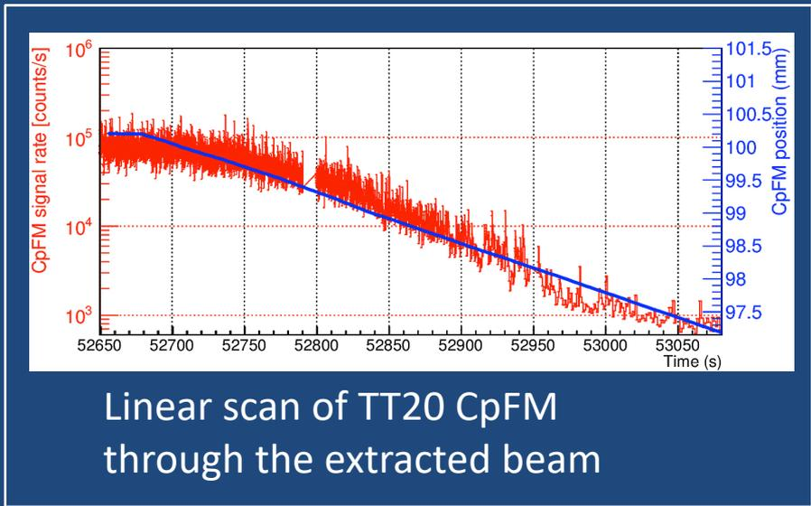
Linear scan of TT20 CpFM through the extracted beam
